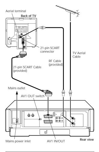
It's essential that your video recorder be properly connected. Follow these steps carefully. THESE STEPS MUST BE COMPLETED BEFORE ANY VIDEO OPERATION CAN BE PERFORMED.
